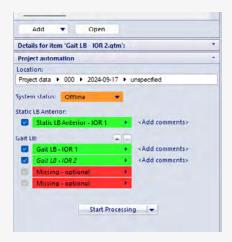
Color coded buttons make it easy to track the progress of a session. When the required trials are captured, analysis is as simple as clicking the "Start Processing" button.
