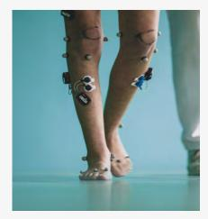
The Qualisys Clinical System can be extended with selected, Delsys, Noraxon, or Cometa EMG systems. EMG data is recorded and processed with the motion capture data, and all results are contained in a single report.
